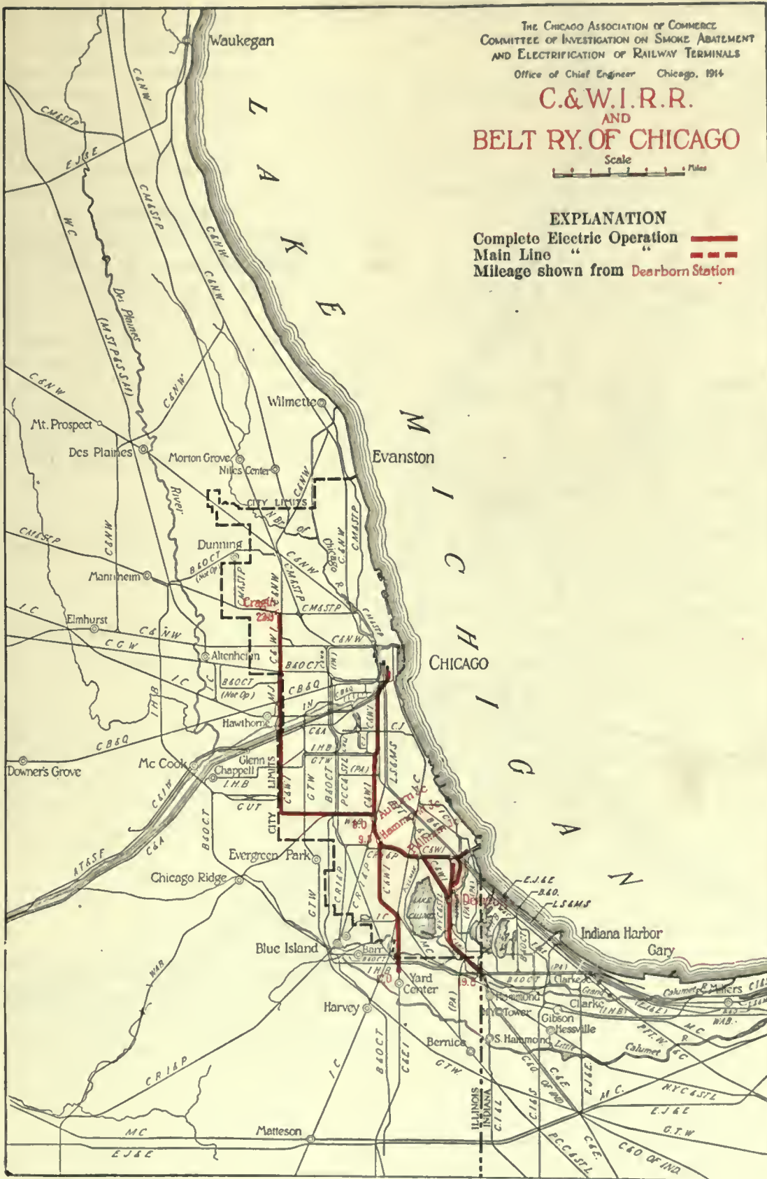
FIG. 553. TRACKAGE TO BE ELECTRIFIED BY THE CHICAGO & WESTERN INDIANA RAILROAD AND THE BELT RAILWAY OF CHICAGO
